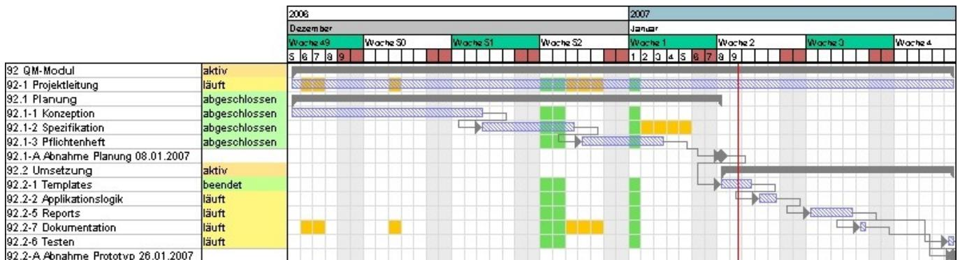
**Gantt chart (= Gantt diagram)** A Gantt chart is a diagram to visualize the time schedule of a [project](#). The duration of a [workpackage](#) or project is symbolized by the length of the bar in the time axis. The bars can include both actual and target data. Events or [milestones](#) are represented as points in time. In Projectile, processes are visualized in [project evaluation](#).
